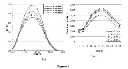
During the night, the temperature of the absorber-1 decreased and the convective heat exchange between the absorber-1 and the airflow became lower, which leads to decrease the average temperature in the drying cabinet to 298 K at midnight. This temperature is weak to ensure drying during nighttime. At the same instant, the temperature of the granite is relatively high, which ensures an extended operation of the chimney even there is no sun because of the heat stored during the day.
